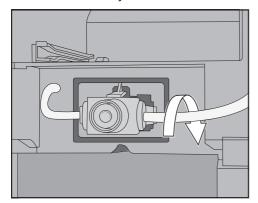
**Useful tip:** If necessary, turn the milk pipework on the right towards the back.
