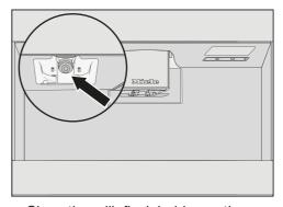
Clean the milk flask holder on the coffee machine with a damp cloth.
