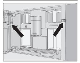
Secure the coffee machine to the side walls of the housing unit using the screws supplied. Tighten the screws by hand.
