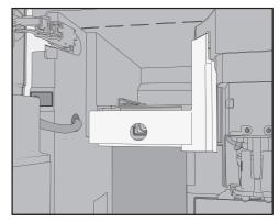
Remove the milk valve cover: on the top right there is a pin which enables you to swing open the cover.
