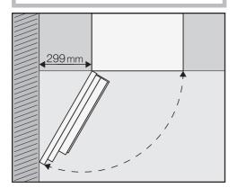
Check whether there is a gap of at least 299 mm between the wall or similar and the coffee machine so that the door can
