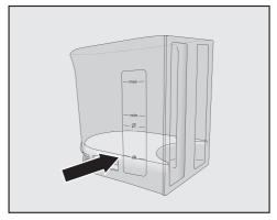
■ Fill the water container to the ////\ marker with lukewarm water and stir the solution.
