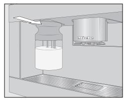
Push the milk flask into the coffee machine until it clicks into place.
