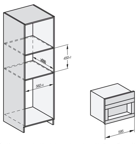
Combination with other Miele built-in appliances is possible. If the coffee machine is to be built in above another appliance, there must be a full-width, closed shelf between them. When built in above a warming drawer, a closed shelf is not needed.
