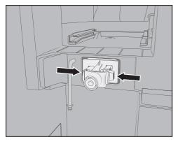
Push the catches on the left and right of the milk valve holder and pull the holder forwards to remove.
